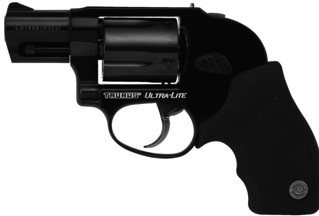
Figure 4.7 Taurus Model 851 Ultra Lite is capable of single- or double-action operation. The hammer is shrouded by the frame, but there is a small textured appendage that permits thumb cocking for single-action firing if desired. (Image courtesy of Taurus International Manufacturing, Inc.)
